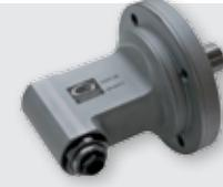
This is a range of heads for traditional machine tools with flange attachment. The T-slot on the universal flange facilitates positioning the head 360° around its vertical axis. The modular system makes it possible to extend the length of the body by adding a spacer. The extension spacer, drive tapers and universal flange are modular and therefore interchangeable among all the heads of similar size.
