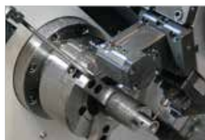
Chuck Air Blow (Upper Chuck)
